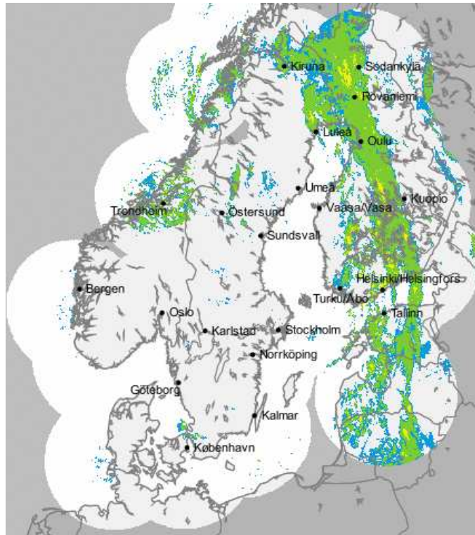
Figure 2: Sample radar image showing the NORDRAD coverage area.
