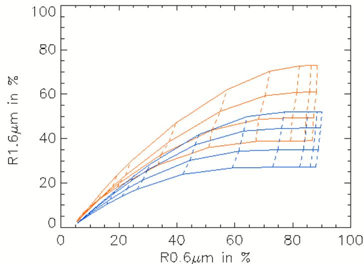
*Figure 39 Illustration of the simulation of 0.6 $\mu\text{m}$  and 1.6 $\mu\text{m}$  cloud reflectances for a selection of water (in orange) and ice (in blue) cloud models for a given oceanic location (fixed viewing angles and surface cloud-free reflectances).*
