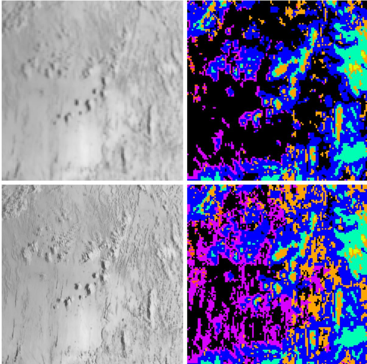
*Figure 22 Sunlint with trade-wind convective low clouds over Indian Ocean, 8 September 2009, 04h00UTC, (120x120 at low resolution SEVIRI scale). Top left: 0.8  $\mu\text{m}$  visible reflectance; top right: v2009 cloud type; bottom left: HRV reflectance; bottom right: v2010 cloud type*
