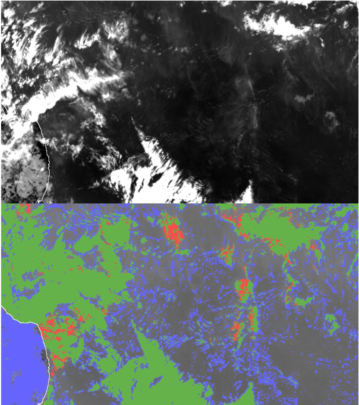
*Figure 12 Meteosat-10, 20 March 2013 15h00 UTC ; (top) enhanced T10.8 (top) ; (bottom) red pixels correspond to those flagged as cloud by the prototyped RTTOV-based test of T108, green corresponds to pixels detected both by prototype and operational SAFNWC, and blue are detections by other operational SAFNWC test*
