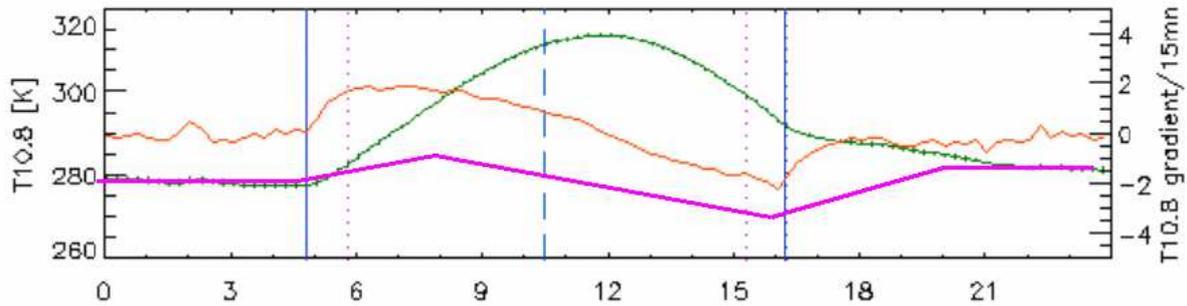
Figure 16 graphical illustration of DT10.8 threshold over land (pink) for a 24h period labelled in UTC time, sunrise and sunset are vertical solid blue line, compared with a real T10.8 cycle (green) and its gradient (orange) for a 15 minute interval
