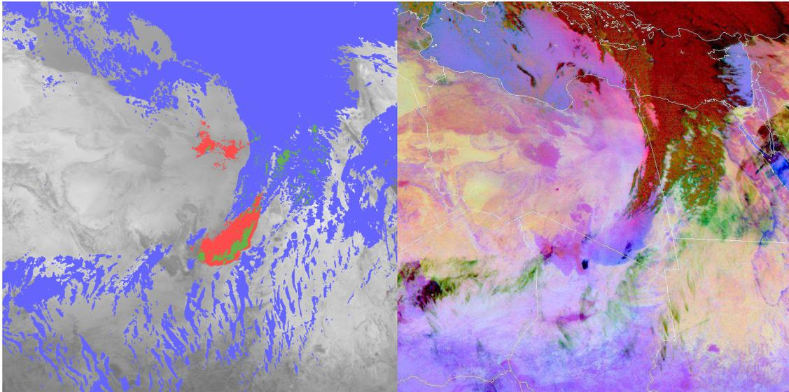
*Figure 14 Meteosat-10, 22 February 2013 00h00 UTC ; Prototype T8.7-T3.8 direct thresholding (left), red pixels correspond to those flagged as cloud by the prototyped RTTOV-based test of T8.7-T3.8, green corresponds to pixels detected both by prototype and operational SAFNWC, and blue are detections by other operational SAFNWC test, grey pixels are T8.7 (warm is dark); EUMETSAT dust RGB (right)*
