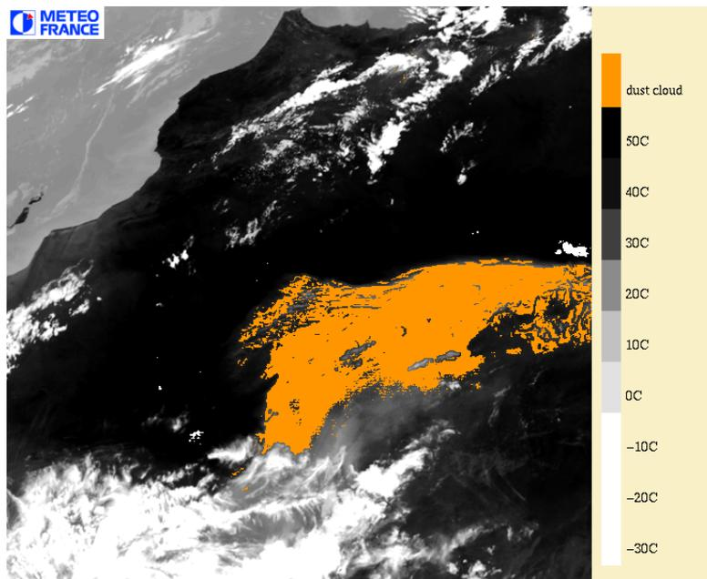
Figure 30: Example of SEVIRI dust cloud flag superimposed on a 10.8 $\mu$ m infrared image: dust cloud over North Africa on 14<sup>th</sup> July 2003 at 13h00 UTC.
