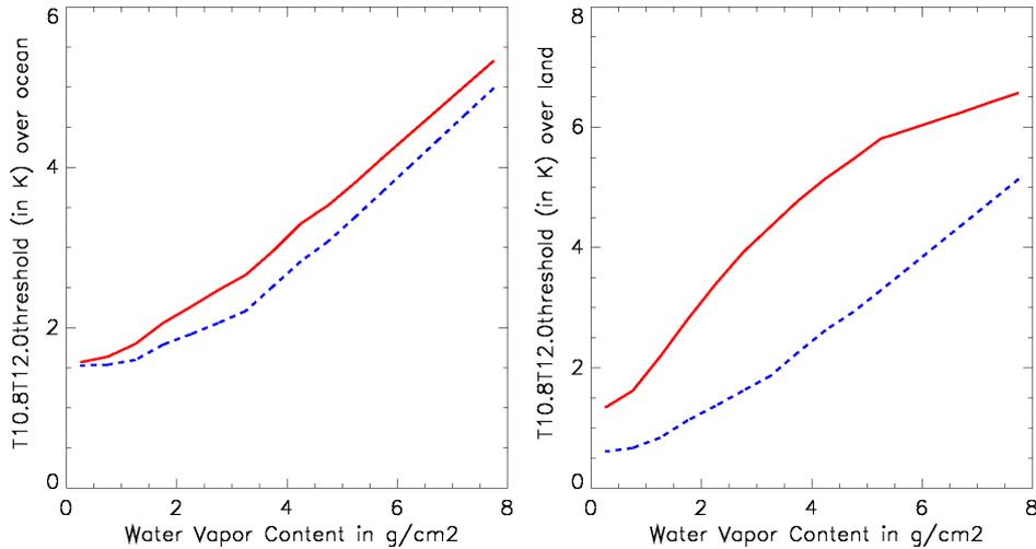
Figure 2: Illustration of  $T_{10.8T_{12.0}}\text{threshold}$  for a satellite zenith angle of 48 degrees. Over Ocean, blue and red curve correspond to cold and warm seas. Over Land, blue and red curves correspond to nighttime and daytime conditions
