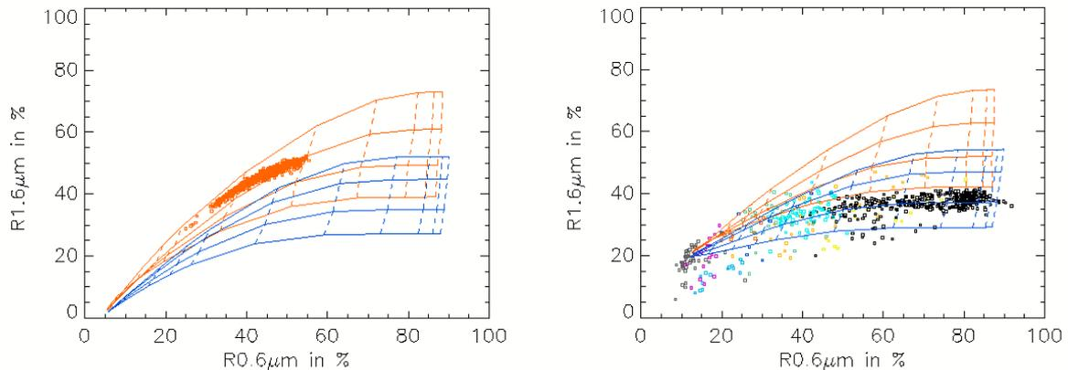
*Figure 40 Illustration of the cloud phase retrieval using 0.6µm and 1.6µm reflectances. Cloud measurements (coloured using CT cloud type colors, except white color replaced by black) are superimposed to simulated curves. Left: for a maritime stratocumulus cloud; right: for a convective system over the Pyrenees.*
