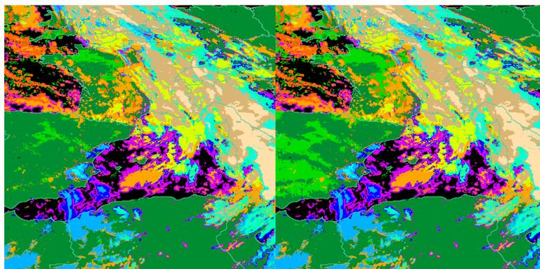
*Figure 19 Illustration of spatial expansion restoration and stationary cloud restoration displayed in light green in CT picture (right) compared with stationary clouds restoration only (left), MSG2 on 25 September 2006, 06h30 UTC*
