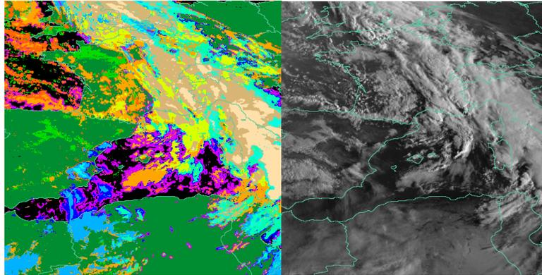
*Figure 17 Illustration of stationary clouds restoration displayed in light green in CT picture (right) compared with BRF 0.6 (left) MSG2 on 25 September 2006, 06h30 UTC*
