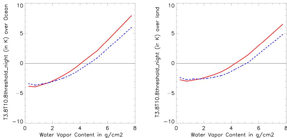
Figure 4: Illustration of  $T_{3.8}T_{10.8}threshold\_night$  for a satellite zenith angle of 48 degrees. Blue and red curve correspond to cold and warm vegetated surfaces.
