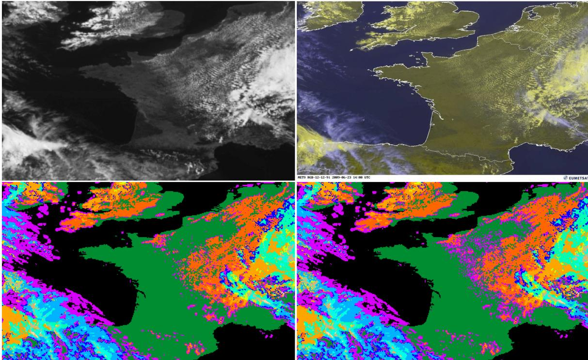
*Figure 23 Fair-weather cumulus in subsident air over western Europe, 23 June 2009, 14h00UTC, (1270x770 at SEVIRI low resolution scale). Top left: enhanced 0.6 μm visible reflectance; top right: EUMETSAT RGB (12-12-9); bottom left: v2009 cloud type; bottom right: v2010 cloud type*
