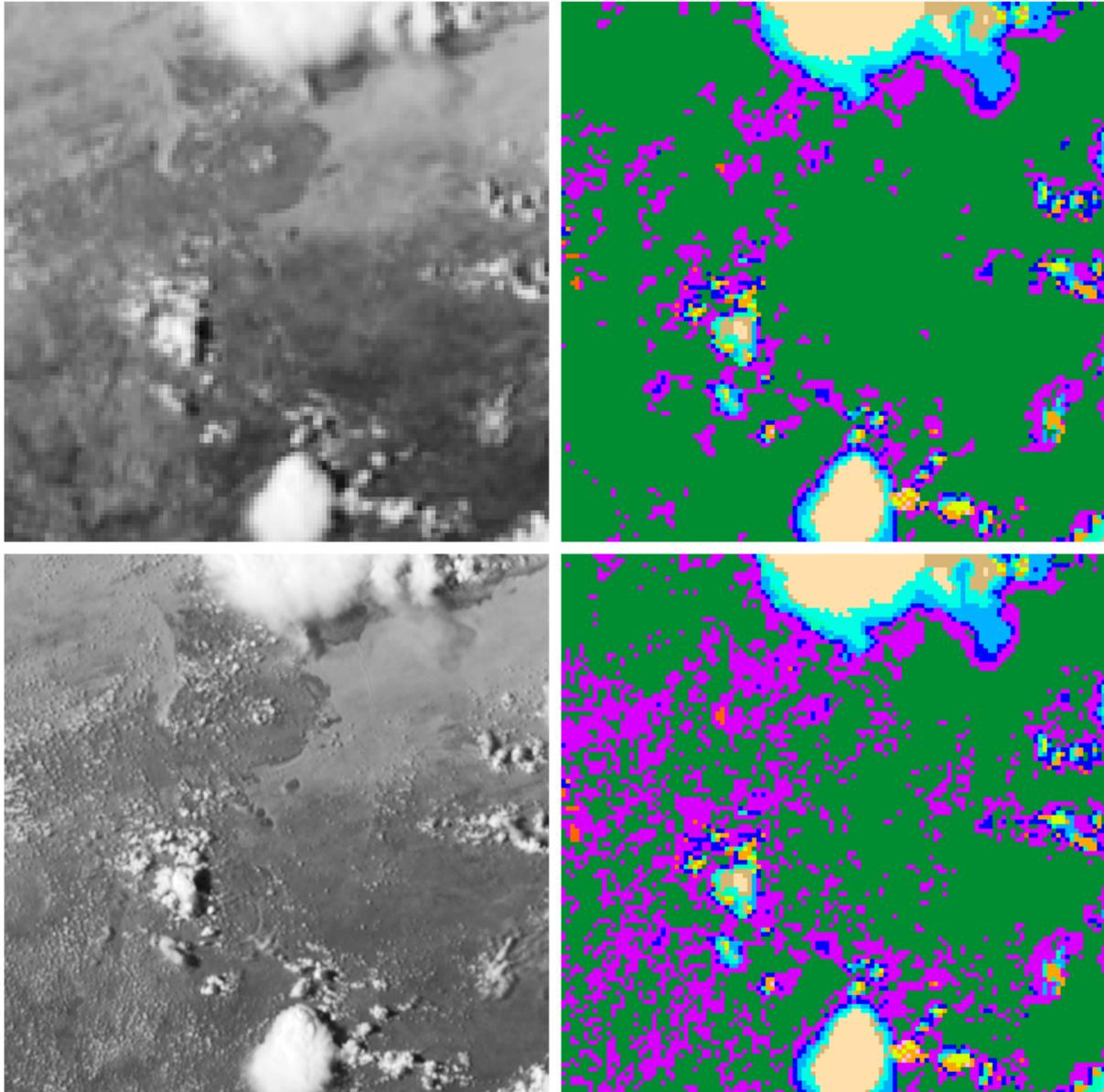
*Figure 24 Heterogeneous convection over complex terrain in Mauritania, 8 September 2009, 15h00UTC, (120x120 at low resolution SEVIRI scale). Top left: 0.6  $\mu\text{m}$  visible reflectance; top right: v2009 cloud type; bottom left: HRV reflectance; bottom right: v2010 cloud type*
