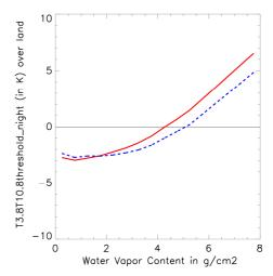
Figure 4: Illustration of T3.8T10.8threshold\_night for a satellite zenith angle of 48 degrees. Blue and red curve correspond to cold and warm vegetated surfaces.
