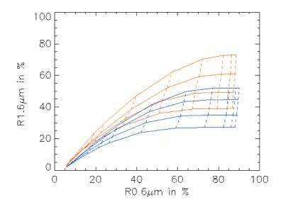
Figure 39 Illustration of the simulation of 0.6 \( \mu \) and 1.6 \( \mu \) m cloud reflectances for a selection of water (in orange) and ice (in blue) cloud models for a given oceanic location (fixed viewing angles and surface cloud-free reflectances).
