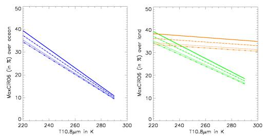
Figure 33: Illustration of MaxCiR06 over Ocean and over Land. Solar zenith angles (30 and 70 degrees), azimuth difference (0 and 90 degrees). In green over vegetated areas, in brown over desert
