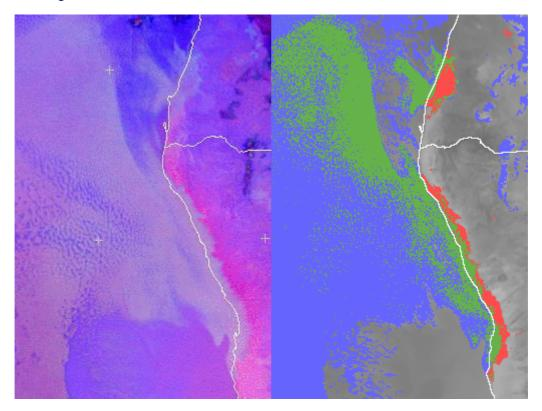
Figure 13 Meteosat-10, 2 March 03h00UTC; EUMETSAT Fog RGB depicting low cloud spreading over Namib desert (left), Prototype T8.7-T3.8 direct thresholding (right), red pixels correspond to those flagged as cloud by the prototyped RTTOV-based test of T8.7-T3.8, green corresponds to pixels detected both by prototype and operational SAFNWC, and blue are detections by other operational SAFNWC test, grey pixels are T3.8 (warm is dark)
