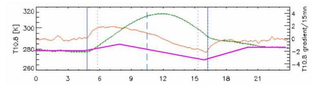
Figure 16 graphical illustration of DT10.8 threshold over land (pink) for a 24h period labelled in UTC time, sunrise and sunset are vertical solid blue line, compared with a real T10.8 cycle(green) and its gradient (orange) for a 15 minute interval
