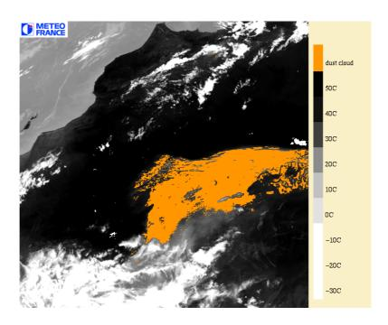
Figure 30: Example of SEVIRI dust cloud flag superimposed on a 10.8µm infrared image: dust cloud over North Africa on 14<sup>th</sup> July 2003 at 13h00 UTC.
