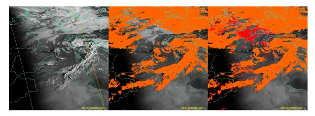
Figure 20 31 August 2007, 05h30 UTC METEOSAT 9 left: Normalized SEVIRI 0.6 with limits of transition area (yellow) and 1h earlier (green) centre: SAFNWC/MSG v2.0 cloud mask (orange) superimposed with SEVIRI 0.6 right: same as centre with new twilight detection (red)
