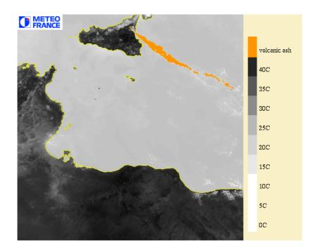
Figure 31: Example of MODIS volcanic ash cloud superimposed on a 10.8 µm infrared image: Etna eruption on 22th July 2001 at 9h55 UTC.
