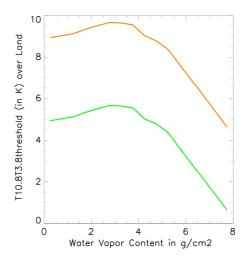
Figure 5: Illustration of T10.8T3.8threshold for a satellite zenith angle of 48 degrees. Over Land, green and brown curves correspond to vegetation and desert.
