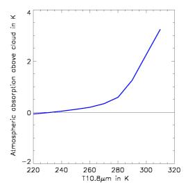
Figure 35: Climatological atmospheric absorption used to compute cloud top temperature from 10.8 µm brightness temperature
