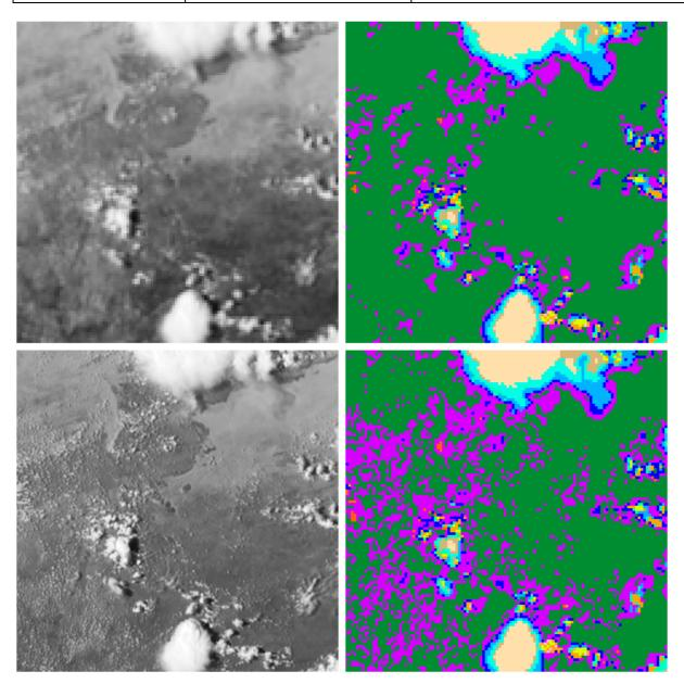
Figure 24 Heterogeneous convection over complex terrain in Mauritania, 8 September 2009, 15h00UTC, (120x120 at low resolution SEVIRI scale). Top left: 0.6 µm visible reflectance; top right: v2009 cloud type; bottom left: HRV reflectance; bottom right: v2010 cloud type
