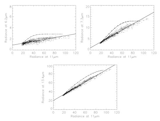
Figure 37: Illustration of the  $H_2O/IRW$  intercept method with SEVIRI radiances (expressed in mWm<sup>2</sup> sr<sup>-1</sup>cm).
