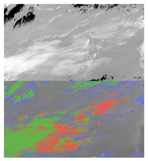
Figure 11 Meteosat-10, 3 March 2013 21h00 UTC; (top) enhanced T10.8-T3.8 with low clouds appearing clear gray, sea in intermediate gray and high clouds dark; (bottom) red pixels correspond to those flagged as cloud by the prototyped RTTOV-based test of T3.8, green corresponds to pixels detected both by prototype and operational SAFNWC, and blue are detections by other operational SAFNWC test, grey pixels are T39 (warm is dark)
