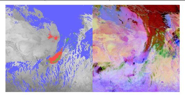
Figure 14 Meteosat-10, 22 February 2013 00h00 UTC; Prototype T8.7-T3.8 direct thresholding (left), red pixels correspond to those flagged as cloud by the prototyped RTTOV-based test of T8.7-T3.8, green corresponds to pixels detected both by prototype and operational SAFNWC, and blue are detections by other operational SAFNWC test, grey pixels are T8.7 (warm is dark); EUMETSAT dust RGB (right)
