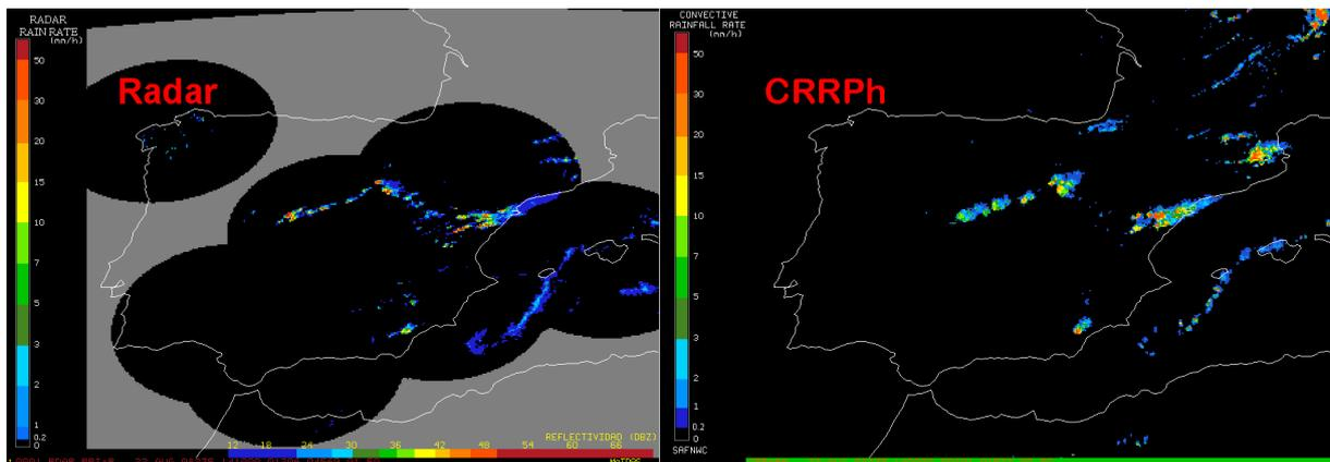
Figure 30. Visual comparison between radar (PPI) and CRR-Ph on 22<sup>nd</sup> August 2008 at 14:00UTC
