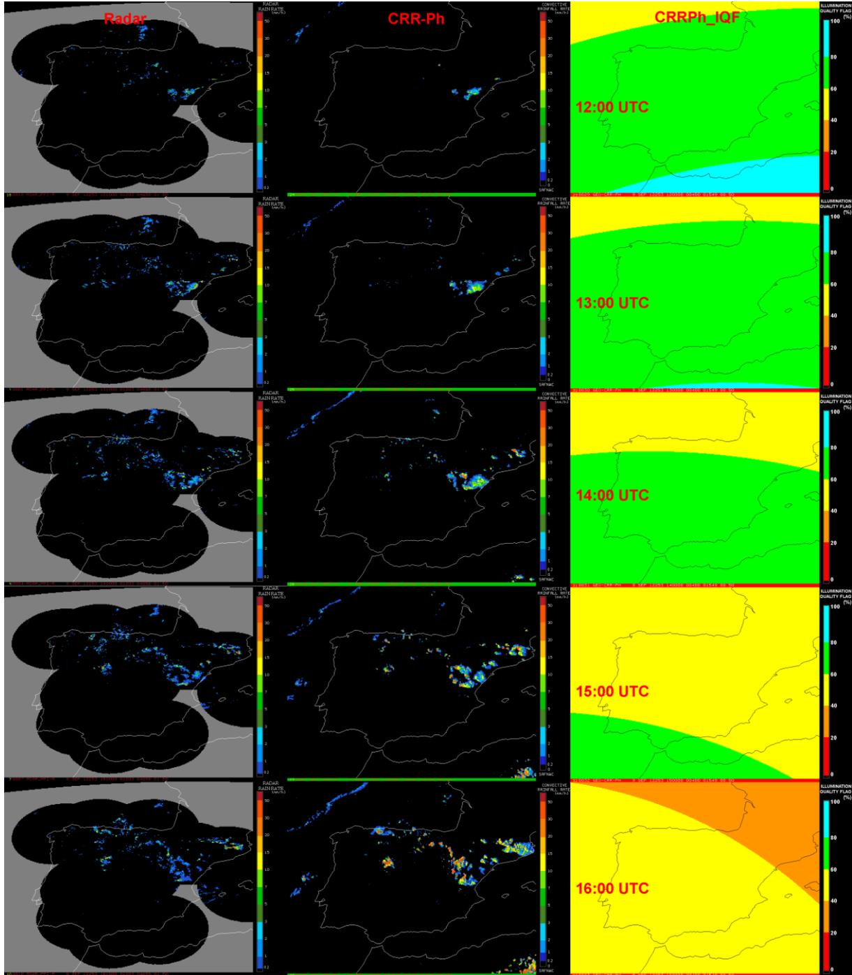
Figure 34. Sequence of radar, CRR-Ph and CRRPh\_IQF images with one-hour time interval that shows the quality degradation of CRR-Ph with poor illumination conditions
