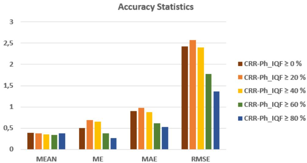
Figure 37. Accuracy measurements for hourly accumulations. Comparison among CRR-Ph product using different CRRPh\_IQF thresholds.
