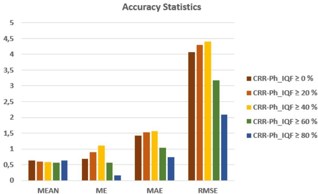
Figure 35. Accuracy measurements for instantaneous rates. Comparison among CRR-Ph product using different CRRPh\_IQF thresholds.
