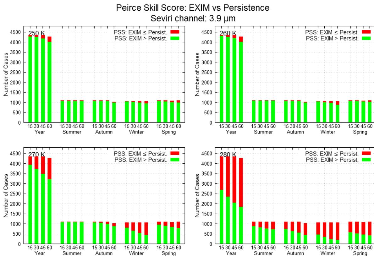
**Figure 46:** SEVIRI channel 3.9 $\mu\text{m}$ . Histogram showing the number of occurrences where the Peirce Skill Score (PSS) of EXIM exceeds (green), or is less than or equal to (red) that for persistence. Each panel corresponds to a threshold value shown in the upper left. Each group of bins represent the data according to season along with a sum over the year, and is separated into the lead times (+15, +30, +45, +60 minutes).
