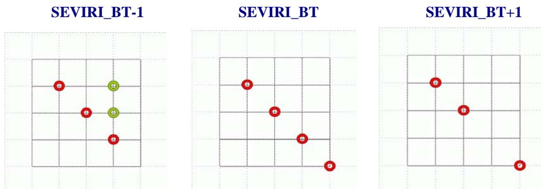
**Figure 3:** Illustration of the diverging counting method. From left to right: Excerpts of the PGE10 grid with modified SEVIRI brightness temperature (-1 Kelvin) test run, reference run and test run with modified SEVIRI brightness temperature (+1 Kelvin) The identified patterns of interest are
